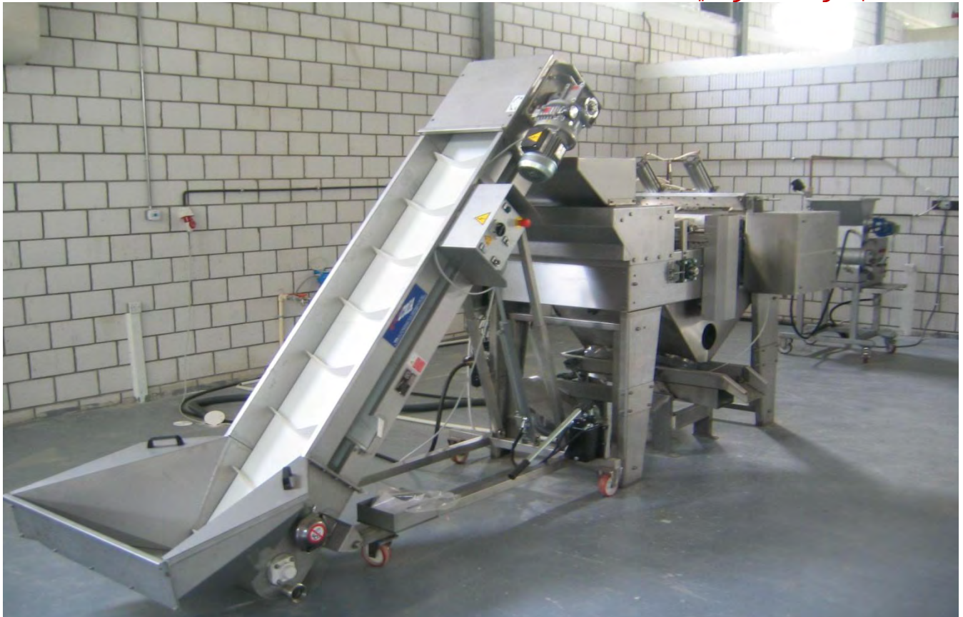
Date Seed Removable Machine 320 date/minute
