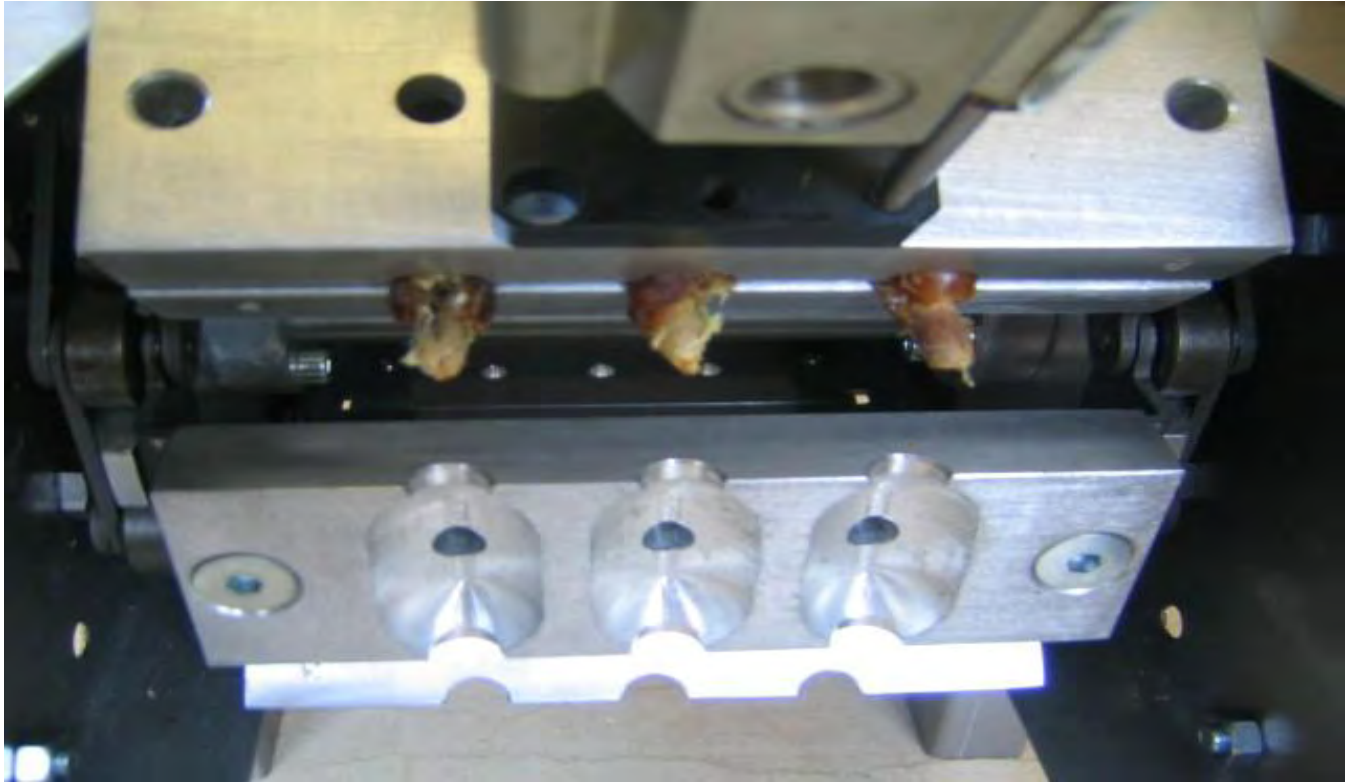
Date Seed Removable Machine 320 date/minute
