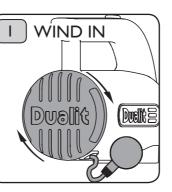
After each use, for easy and tidy storage, wind the power cord into the body of the mixer by turning the swivel base clockwise in the direction shown by the arrow on the mixer body.
