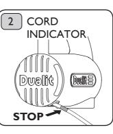
To prevent cord damage always pull power cord out gently. If the cord jams, rotate the swivel base counter clockwise half a turn, then pull out the cord. Do not pull cable past the red indicator on the power cord.
