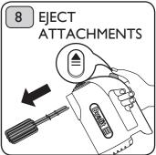
Raise the mixer head and press down on the beater ejector button to eject the beaters. Note: The speed control must be set to '0' to release to beaters.
