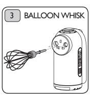
The balloon whisk can fit into either hole. Grasp the handle of the mixer with one hand and the whisk stem with the other hand and insert the whisk with a slight twist and push action until they click in to place.
